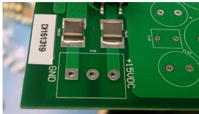
The terminal block is 3 positions, pin 1, towards the board edge, is Ground (GND). Pin 2 is unconnected and must be left unconnected. Pin 3 is the +15 VDC terminal.
