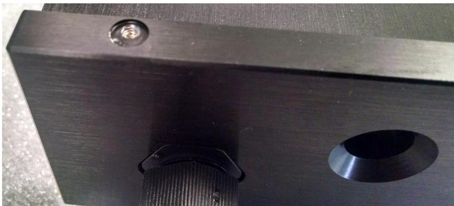
Remove the screw in the center of the housing on the bottom of the Power Supply using a 1/16" Allen wrench.
