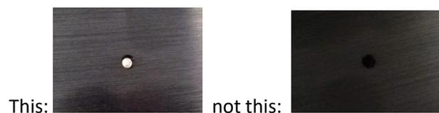
(It will be apparent if it is not mated properly and you will see an empty hole!) Secure the set screws hidden under the feet. Reinstall the screw on the bottom of the supply as well. Once the screws are tight, reattach the rubber feet.
